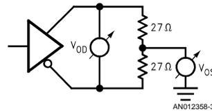
FIGURE 2. Termination Load Configuration
